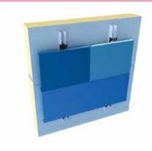
Hybrid FC panel on composite panel: vertical, parallel
