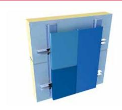
Hybrid FC panel on composite panel: horizontal, parallel
