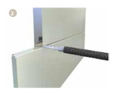
In case of damages, the FC facade enables the exchange of individual panels without the need to dismantle the entire wall cover. The dismantling of a panel can be performed fast and easy by using the especially developed tools of the Kalzip FC tool kit.
