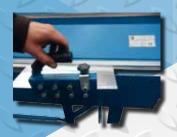
**Welt press / Edge pressing** - convenient and very fast tool for precise pressing of the prefabricated fold in one operation.
