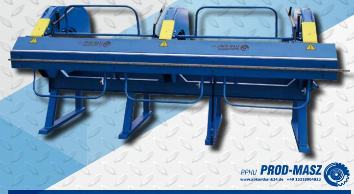
The machines in this group consist of 2 to 6 modules, each separated by 80cm, (supporting arms of the upper beam), which increases stability during the bending process.
