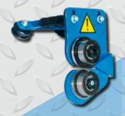
**Rotary shears/cutter NK / 0,8mm** - with adjustable cutting direction and rollers, which are made of high-alloy steel with very high resistance against wear. This allows cutting of sheet over a very long period of time, without re-sharpening. The performance of the cutter is about 40 km of sheet metal with a thickness of 0.5 mm - until the first re-sharpening.
