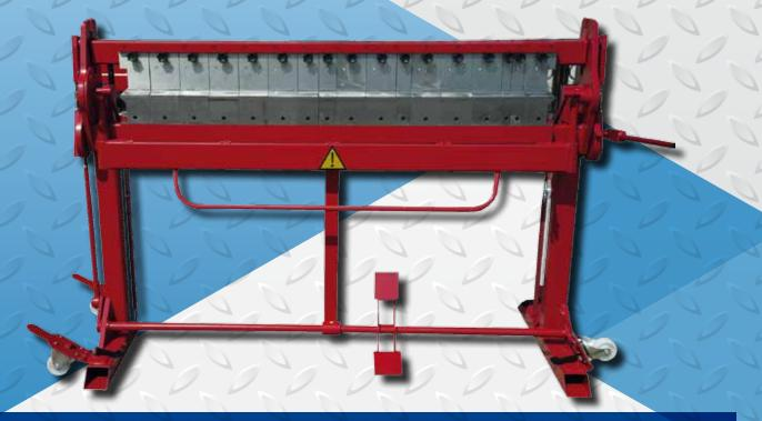
3-fold bending machines with foot control - these machines are equipped with segments in three bars: upper, lower and bending. This makes it possible to bend sheet metal from all sides, e.g. create complex shapes of boxes or objects.
