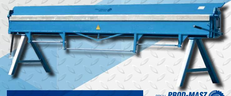
Excellent workmanship and practical solutions are convincing in these bending machines. The bending capacity is sufficient for 0.8 mm thick steel sheets for most applications. The extended legs give these machines a very safe working position and also prevent a rapid "tipping over" during transport.
